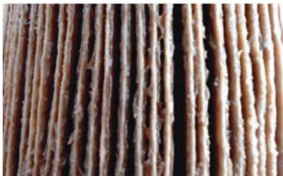
Filter blockage due to high Cloud Point
