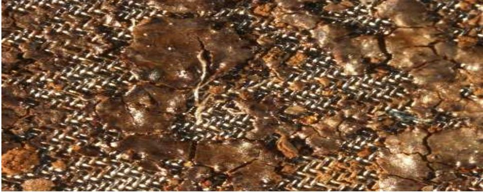
Figure 1: Polyethylene terephthalate separated from a sludge
