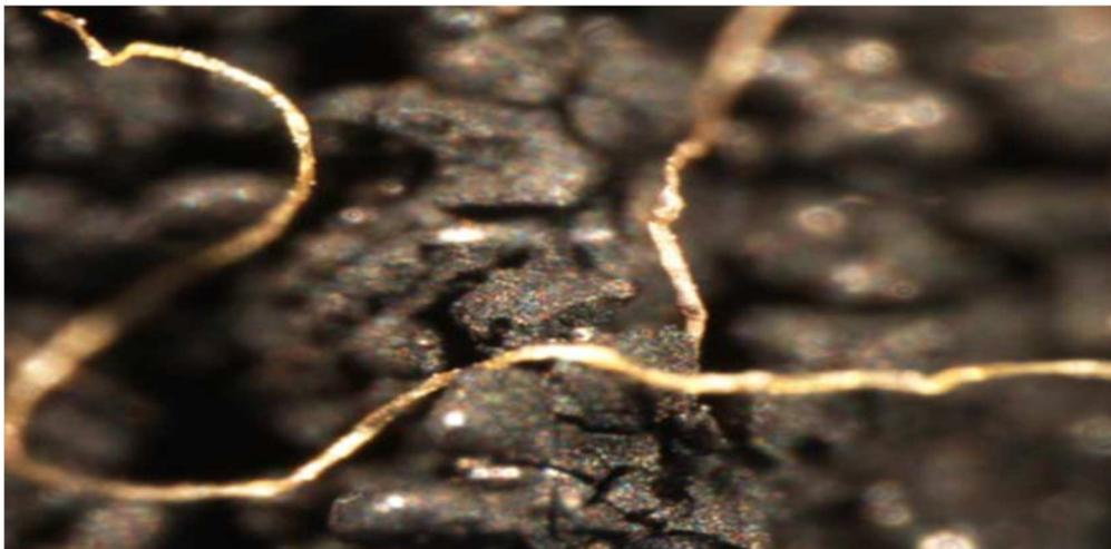
Figure 4: Poly methyl methacrylate and dispersed mix of dark coloured solid masses and inorganic matter separated from a fuel oil
