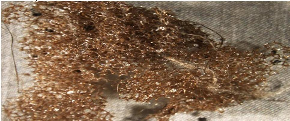
Figure 3: Golden yellow fiber like spongy material separated from a sludge
