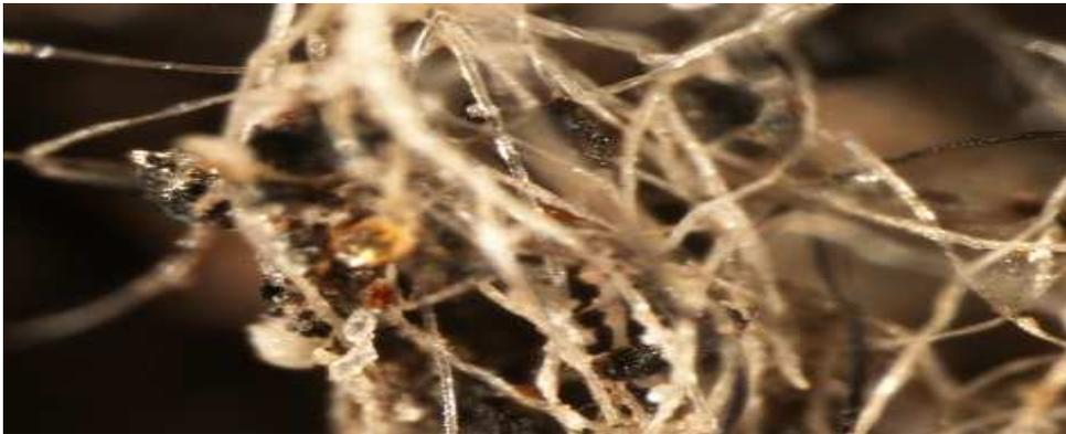
Figure 2: Scattered mix of light and dark coloured solids with few strands of fibers separated from the fuel oil
